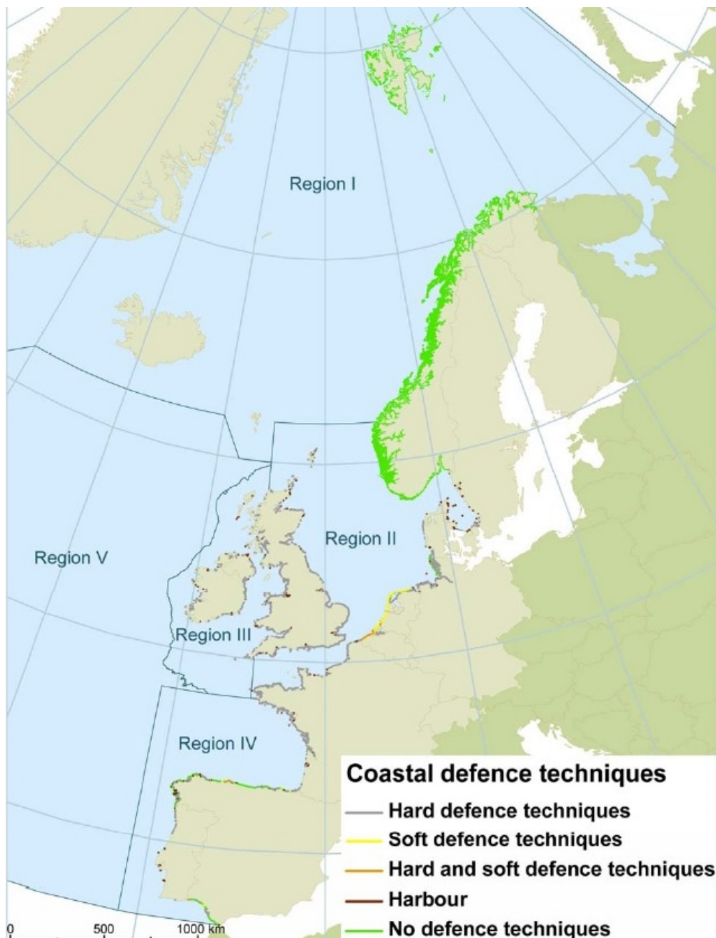
Fig. 4.1 Coastal defence techniques used along the coastline of the OSPAR Maritime Area. (Redrawn from: Govarets and Lauwerts, "Assessment of the impact of coastal defence structures", OSPAR COMMISSION, 2009)
