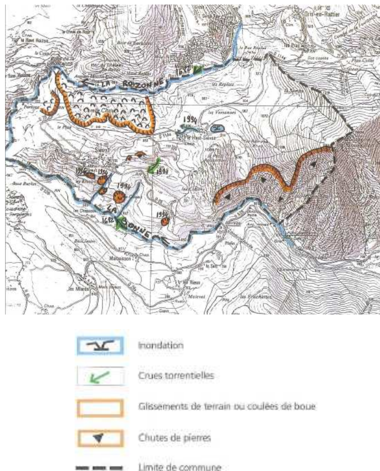
Figure 4-2. Map making an inventory of the past land moves in Sievoz (Isère) (Source: guide méthodologique)
