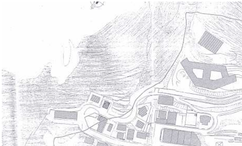
Figure 3-5. Extract from RFMP. The limit that separates the high from the low hazard zone is marked with a dark line.
