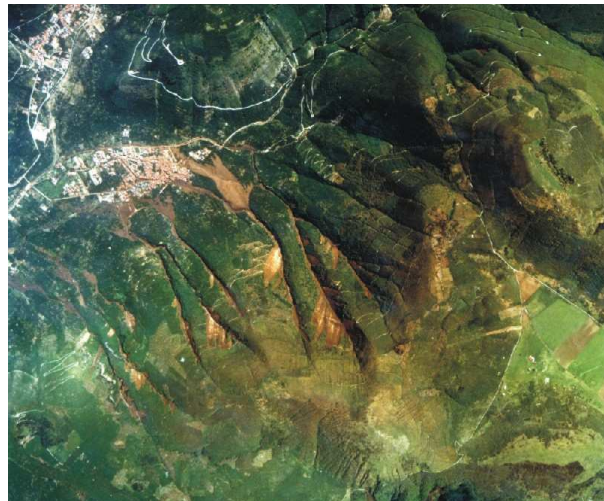
Figure 3-16. Aerial view of the flow-type landslides which occurred at Quindici in may 1998. The landslides covered long distances reached up to 3500-4000 m from the crown zone
