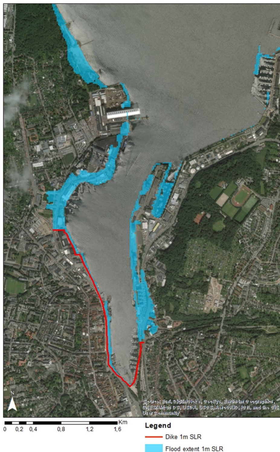
Figure 5: Flood extent in Flensburg based on detailed simulations of the 2017 Axel Storm, assuming a 1-m of SLR and the implementation of a dike protecting parts of the city.
