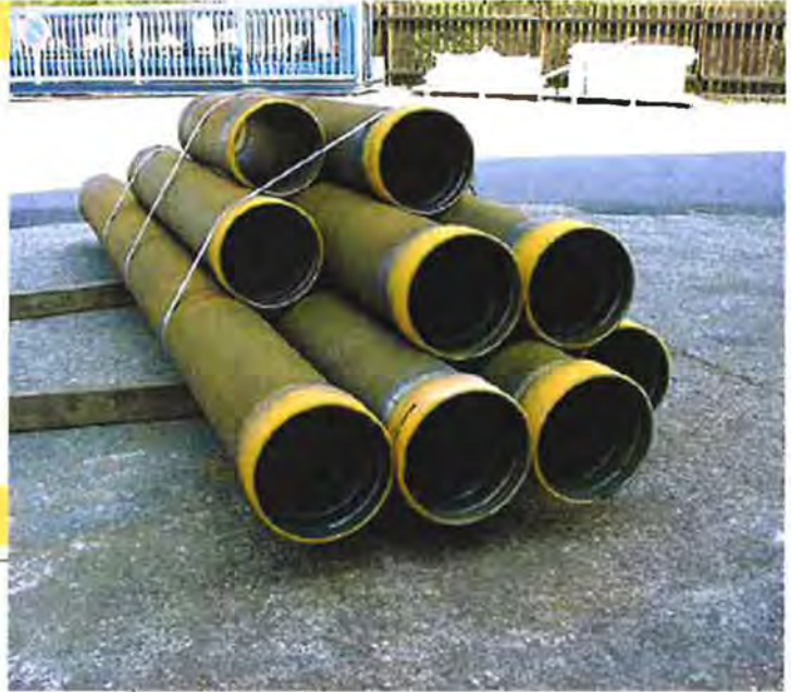
Tremie pipes 250 mm Ø, 2.5 m long, prior to shipment
