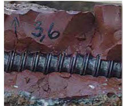
Grout body around TITAN 30/11 injection pile broken away to show completed crack pattern.
